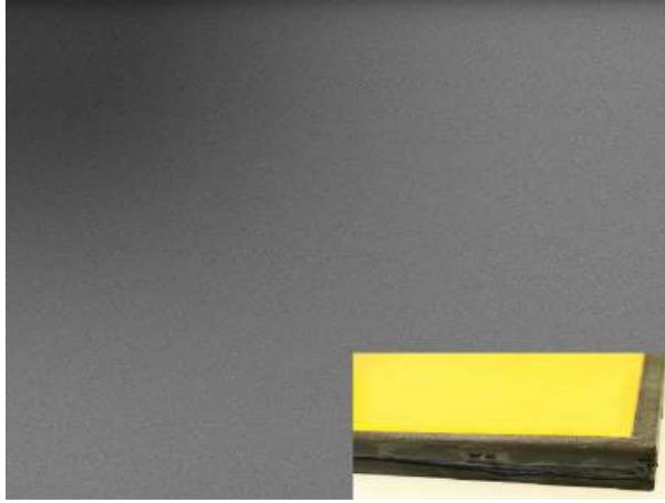
FIG. 61. Cassette that deteriorated over the years (inset), resulting in foggy images (main).
