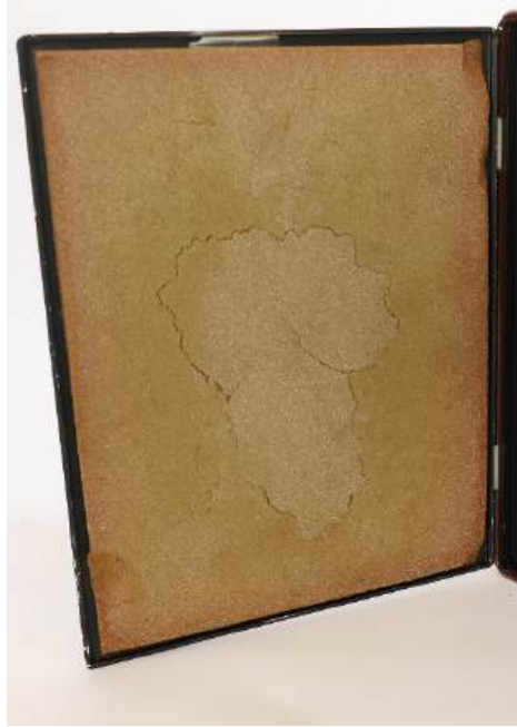
FIG. 62. Cassette with dried out foam causing artefacts because of bad film–screen contact.
