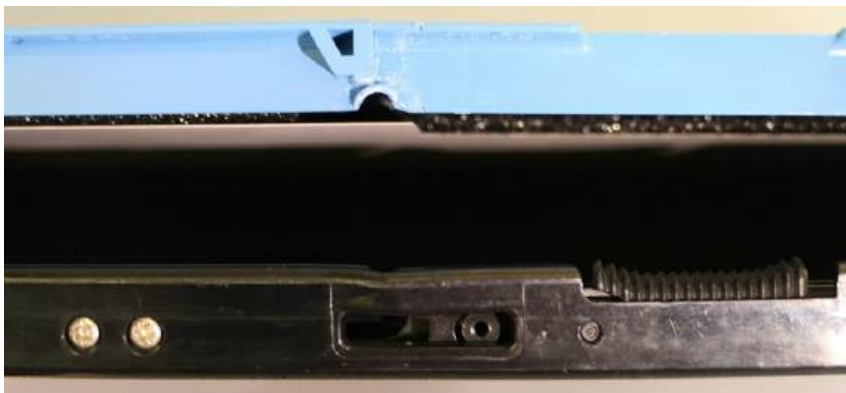
FIG. 59. Cassette on which the latch was stuck and pried open by force.
