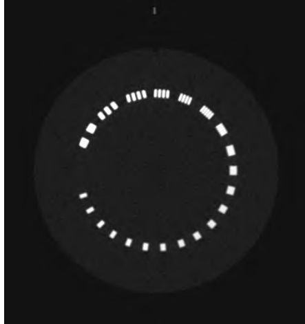
FIG. 55. Bar pattern phantom image with the alignment inset shown at the top.
