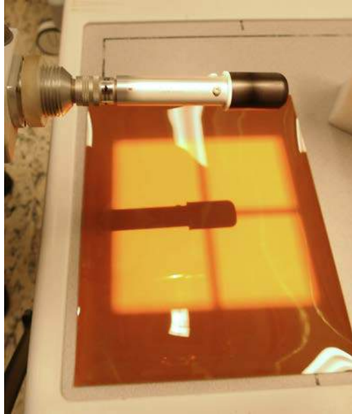
FIG. 11. Set-up using an ionization chamber and a self-developing film to determine the accuracy of the kerma–area product meter.
