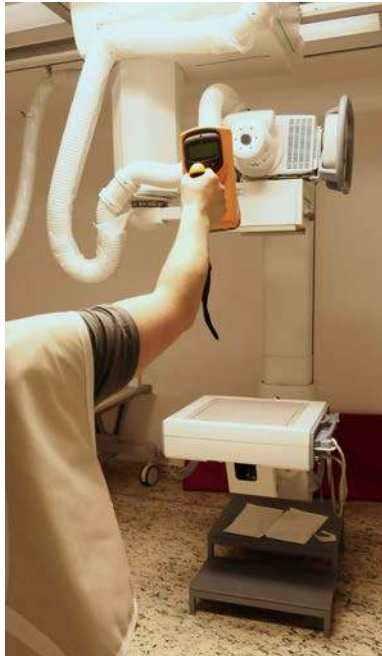
FIG. 13. Measurement of leakage radiation.
