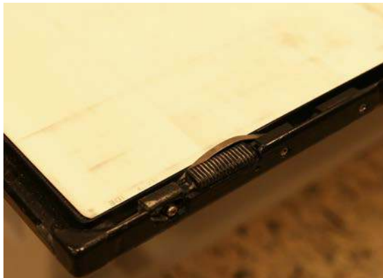
FIG. 7. Defective cassette in which scratches on the screen prevent the processing unit to process it properly.
