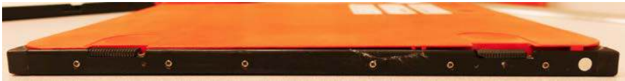
FIG. 6. Defective cassette in which the lock on the right cannot be closed.
