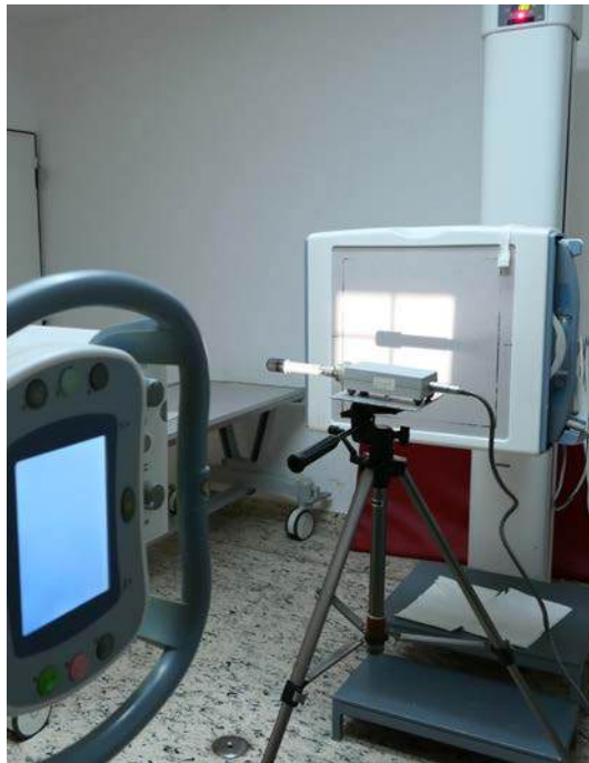
FIG. 10. Set-up with an ionization chamber for measuring air kerma without attenuators.
