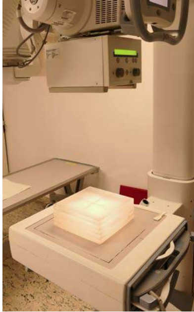
FIG. 4. Set-up for image uniformity test using PMMA.
