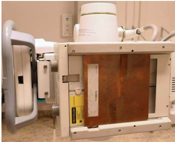
FIG. 5. Arrangement to check the constancy of the automatic exposure control sensor using a copper attenuator.
