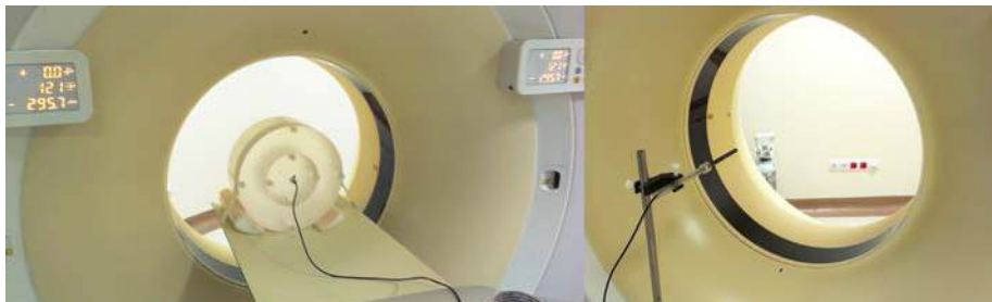
FIG. 56. Set-up for the measurement of dose in a standard CTDI PMMA body phantom (left) and a free-in-air measurement (right).
