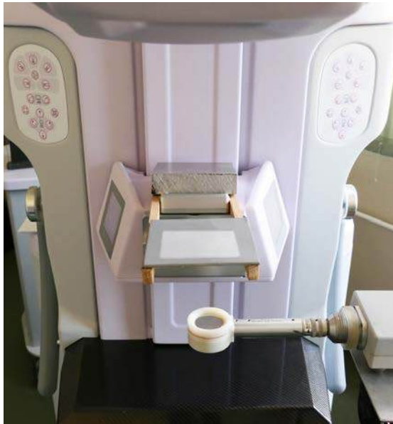
FIG. 35. Set-up for HVL measurement using an Al plate and an ionization chamber.
