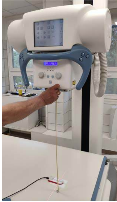
FIG. 9. Set-up for kilovoltage accuracy test using a solid state non-invasive kilovolt meter.
