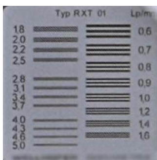
FIG. 16. Image of bar pattern used for the visual determination of the limiting spatial resolution.
