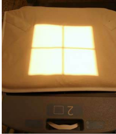
FIG. 17. Digital radiography image receptor covered with a lead apron to test dark noise.
