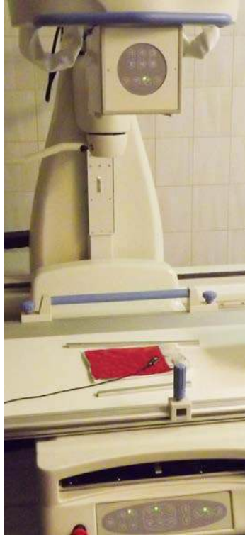
FIG. 20. Set-up for the test of the AEC guard timer, with a lead plate placed beneath the solid state dosimeter.
