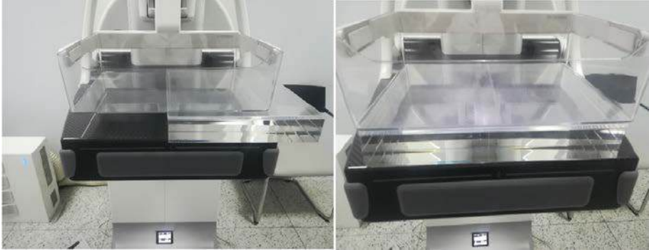
FIG. 44. Phantom set-ups for the creation of ‘ghost 1’ and ‘ghost 2’ images.
