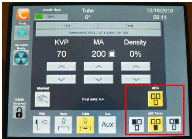
FIG. 8. Control system used for the selection of automatic exposure control ionization chambers (here, the central ionization chamber is selected).
