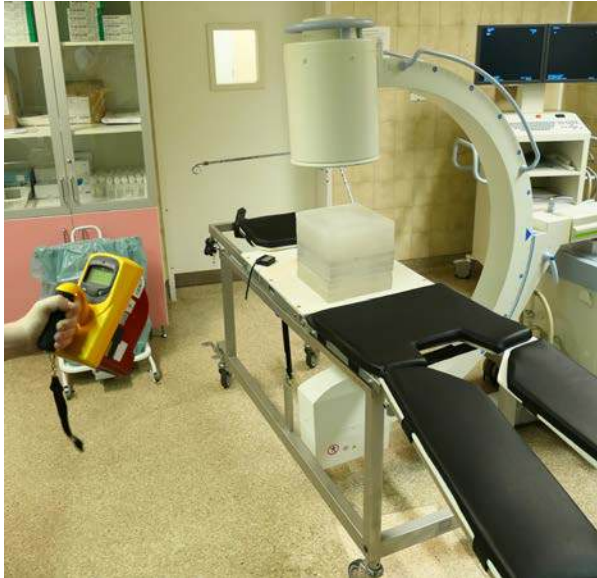
FIG. 14. Set-up for the measurement of scattered radiation around a mobile C arm fluoroscopy unit in the area occupied by staff.
