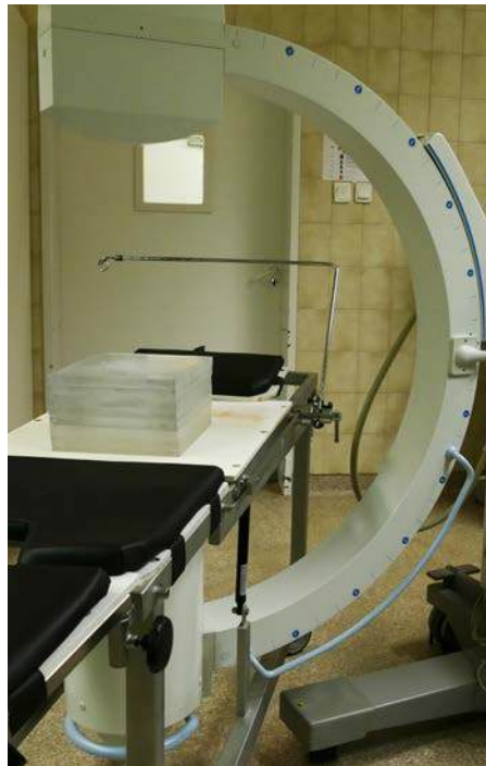
FIG. 22. Simple set-up using PMMA to check the performance of AERC settings.
