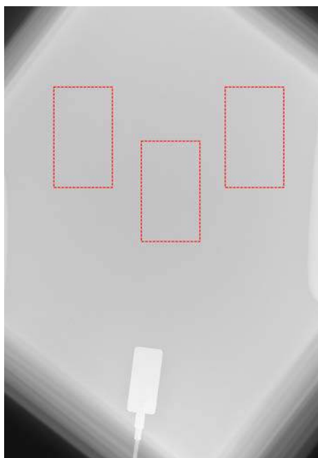
FIG. 12. X ray image showing the set-up for measuring the image receptor dose. A solid state detector and the AEC ionization chamber positions during a measurement under PMMA plates are indicated.
