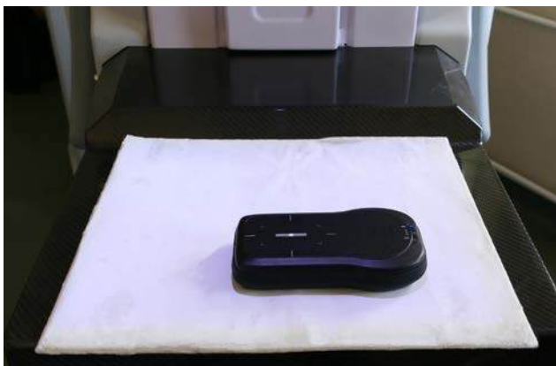
FIG. 34. Set-up for measuring the tube output using a solid state detector.
