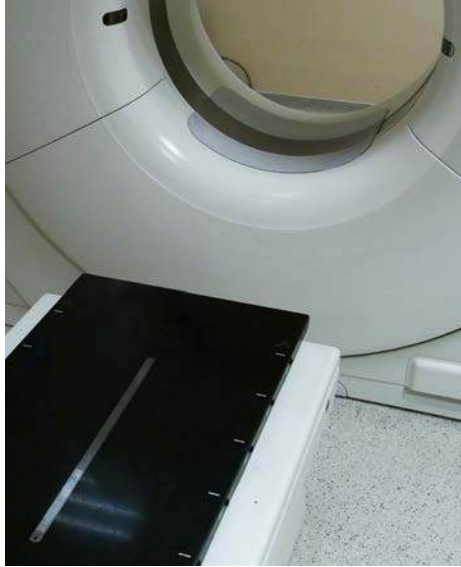
FIG. 48. A 50 cm long steel ruler set to measure the accuracy of the scan projection radiograph.
