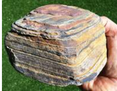
Figure 6.57. Lamination in shale. Each laminae may be an annual cycle of deposition or a seasonal storm flood event (scale is in mm to cm).
