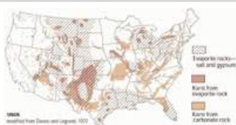
Figure 6.74. Map of the United States showing the location of carbonate rocks in the subsurface. Limestone rock formations occur under about 40% of the continental United States!
