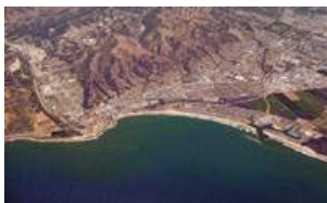
Figure 12.54. The Ventura River (left) supplies massive amounts of sediments to the coast during infrequent floods, then persistent coastal erosion processes take over the action. Construction of the Matilija shut of much of the sediment supply to the coast. The dam is now being removed.
