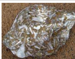
Figure 6.75. Fossiliferous limestone. This sample from Ohio is loaded with ancient coral-like fossils called bryozoans (not corals).
