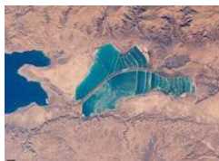
Figure 7.15. Evaporation ponds constructed near the Dead Sea in Jordan are developed to manufacture salt.
