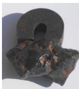
Figure 3.9. An iron-nickel meteorite is magnetic and has a similar density as the metallic core of our planet.
