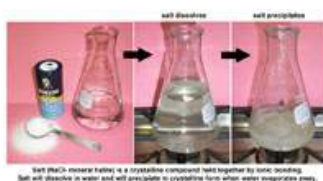
Figure 1.21. Salt crystals are held together by ionic bonds . Salt compounds dissolve in and precipitate from water.
