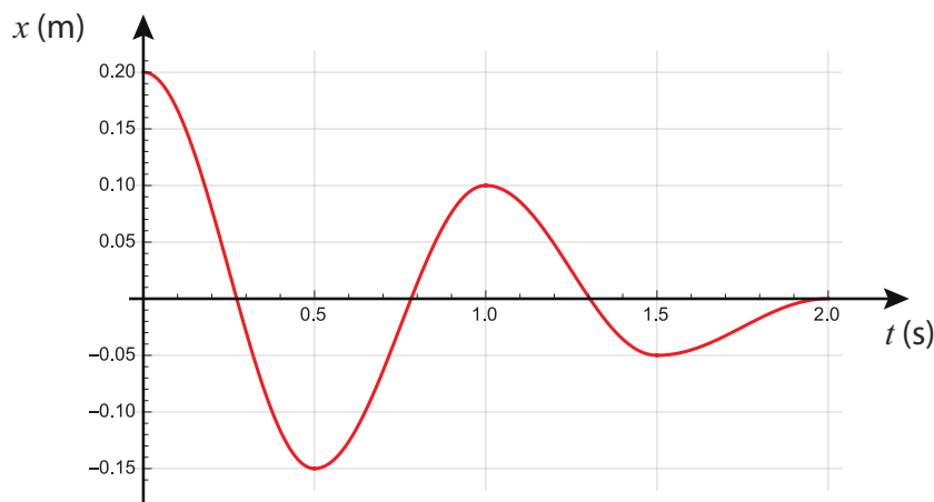
Figure 1.2: A possible position vs. time graph for an object moving in one dimension.
