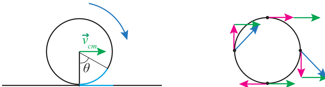
Figure 9.8: Left: illustrating the rolling without slipping condition. The cyan line on the surface has the same length as the cyan-colored arc, and will be the distance traveled by the disk when it has turned through an angle \theta . Right: velocities for four points on the edge of the disk. The pink arrows are the velocities in the center of mass frame. In the Earth reference frame, the velocity of the center of mass, \vec{v}_{cm} , in green, has to be added to each of them. The resultant is shown in blue for two of them.
