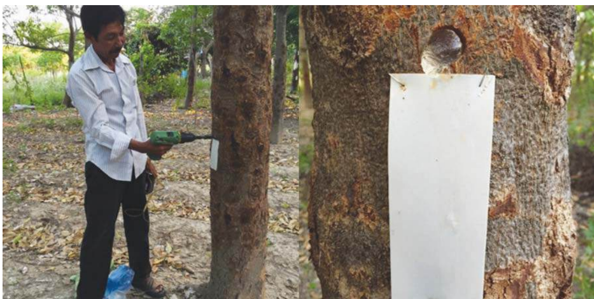
Figure 30. The second tapping method: coring the tree bark
