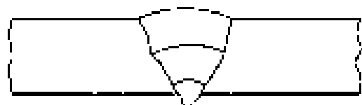
Excess Weld Metal at the Root
