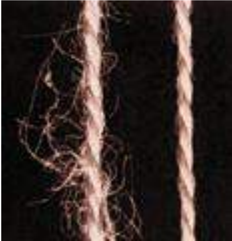
Figure 2 – Singed (Gassed) Yarn – Before and After.
