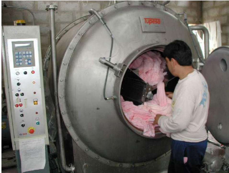
Figure 27 – Typical Rotary Drum Machine.
