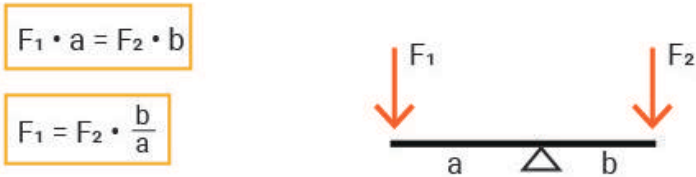
Figure 3-5: Archimedes' principle of the level
