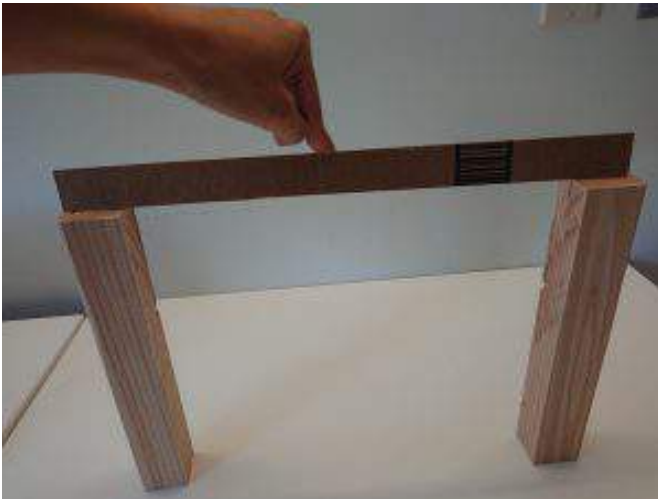
Figure 8-1: Relation between the cross-sectional depth (rise) of a beam and its stiffness
