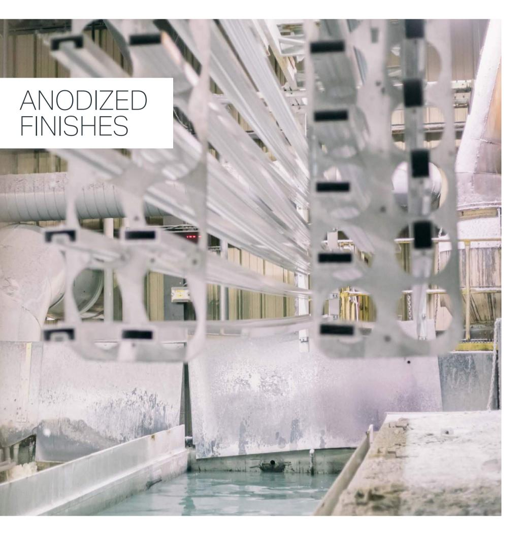
Anodizing is a general term that describes the process of converting the surface of aluminum to aluminum oxide. Under carefully controlled conditions, anodizing produces a uniform oxide coating.
