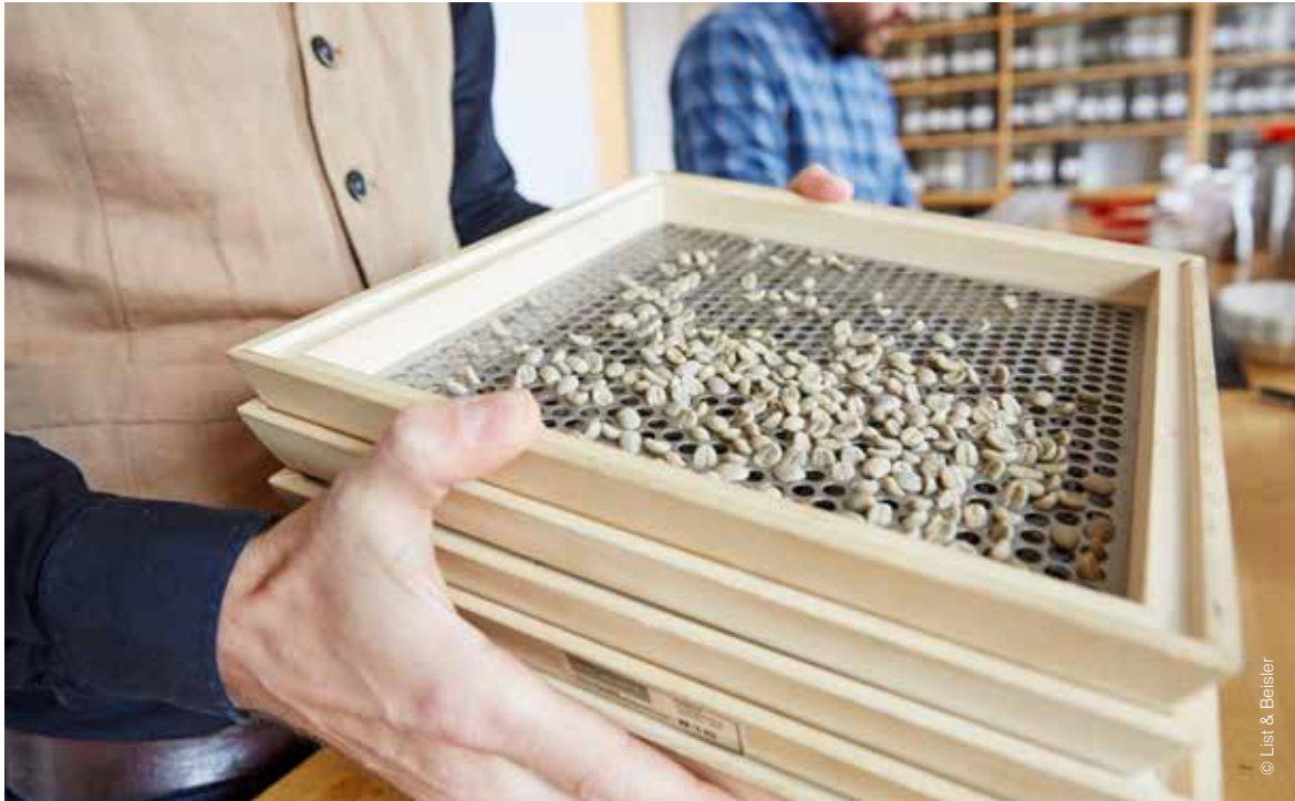
Screens for grading bean size.
