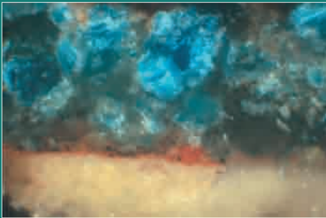
FIGURE 8 Back of a painted wooden chest; Microsample in Osiris' throne; Cross-section of the blue colour; Egyptian blue (> 150 \mu\text{m} ) on red ochre mixed with charcoal (10-15 \mu\text{m} ). On a thick layer of a mixture of calcite and gesso (100-150 \mu\text{m} ). Optical microscope, original size: 0.30 x 0.45 mm
