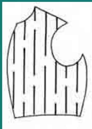
FIGURE 8 The invisible stitches worked in the depth of the fulled wool cloth
