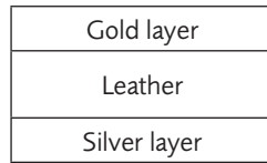
FIGURE 12 Layer structure of the one side gilt, reverse side silver-coated leather strip
