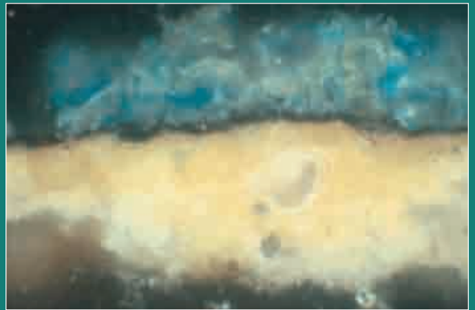
FIGURE 9 Back of a painted wooden chest. Microsample in the blue border: cross-section of the blue colour; Egyptian blue (100 \mu\text{m} ) on a charcoal layer (10 \mu\text{m} ); On a thick layer of a mixture of calcite and gesso (100-150 \mu\text{m} ), Optical microscope, original size: 0.30 x 0.45 mm
