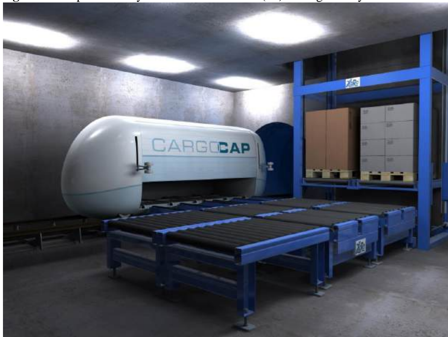
Figure 11: Caps with fully automated horizontal (un)loading conveyors
