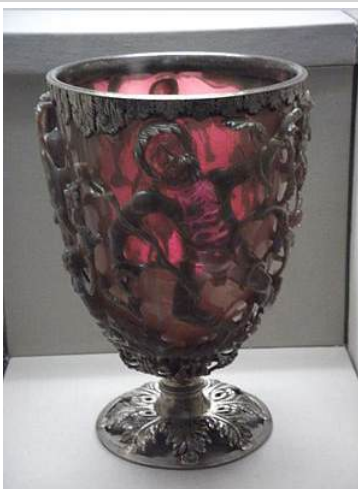
The Lycurgus cup (4th century Roman glass) derives its unique coloration from noble metal nanoparticles. The cup is red in transmitted light and green in scattered (reflected) light.
