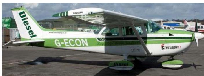
Cessna Centurion 1.7 com motor diesel
