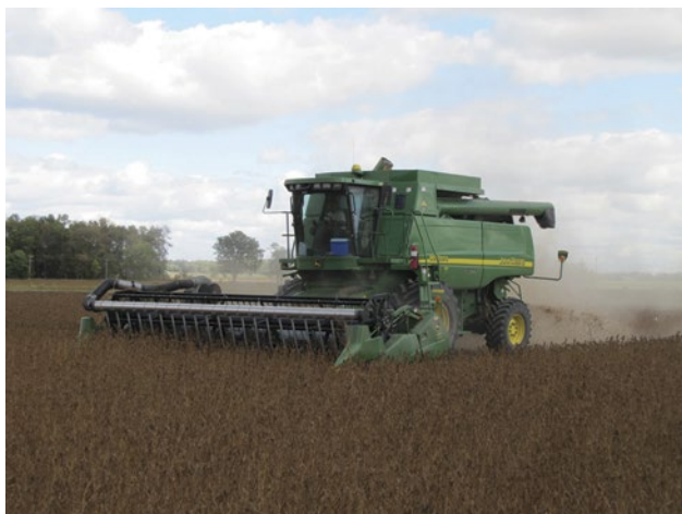
Photo 2–8. Combine with air reel to minimize losses.
