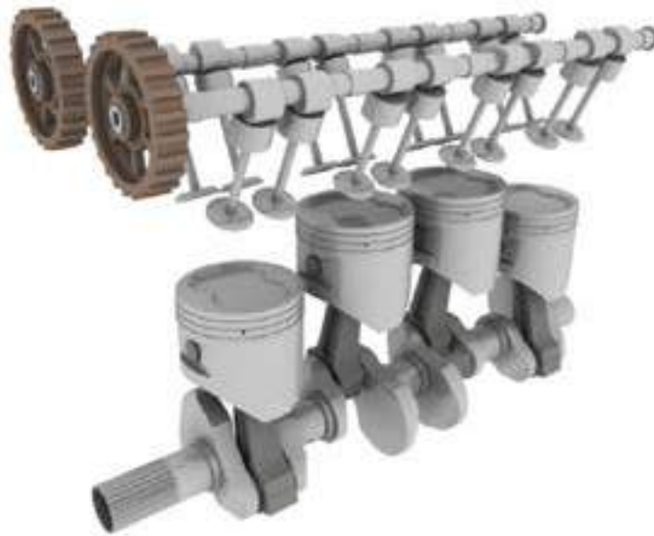
Figure 18 —Diagram of an engine with overhead camshafts, demonstrating valve train components
