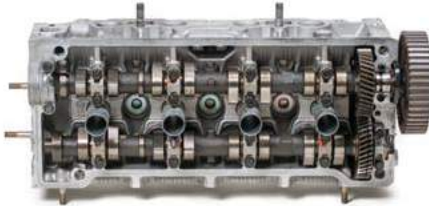
Figure 9 —Top view of cylinder head with camshafts attached
