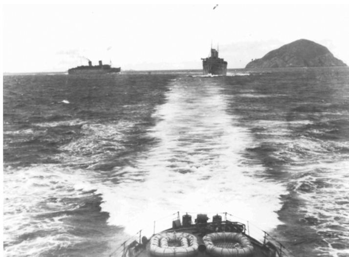
Figure 67: The stern of Sydney in September 1941 showing the location of the two Pattern No. 18 Carley floats with a Pattern No. 20 Carley float inside the starboard No. 18 float [126].
