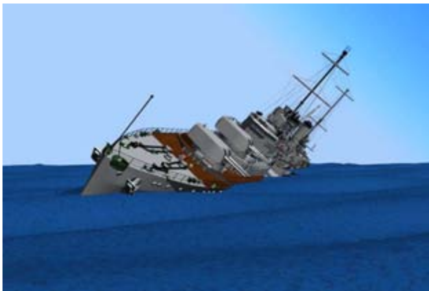
Figure 272 Visualisation of Sydney at a roll angle of approximately 40° in Sea State 3
