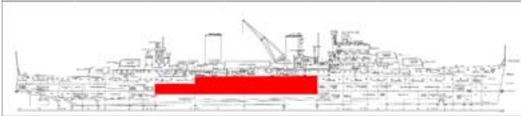
Figure 42: Profile of Sydney showing the extent of ship's side armour [5]
