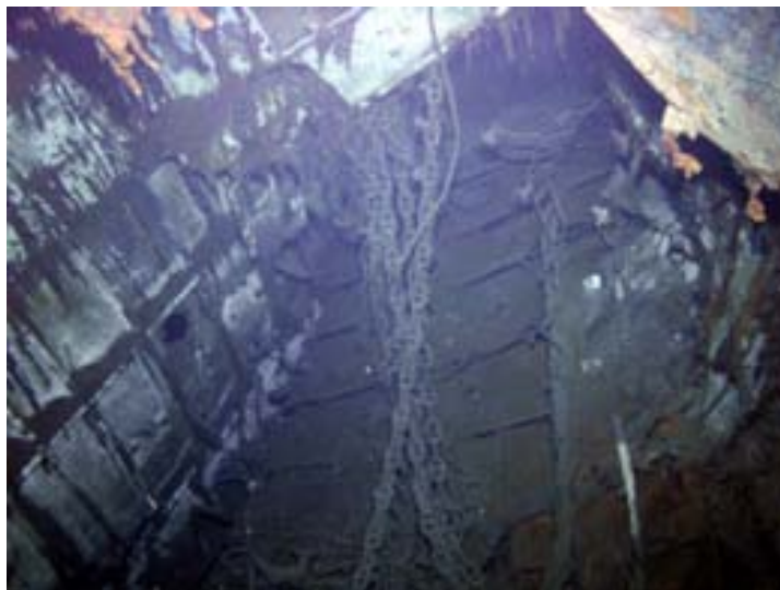
Figure 119: Internals of the bow show collapsed decks and connected anchor chains [175]
