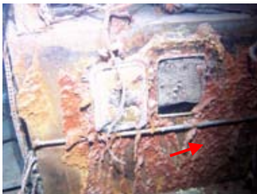
Officer's galley, Forecastle deck (aft - port). Note the rusticles (see arrow).
