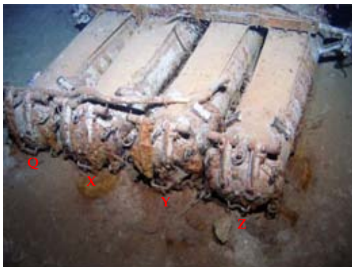
Figure 196: End caps of starboard quad tubes showing embossed lettering [279]
