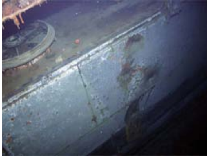
Figure 192: 15 cm shell hits below starboard torpedo mounting ring [276]
