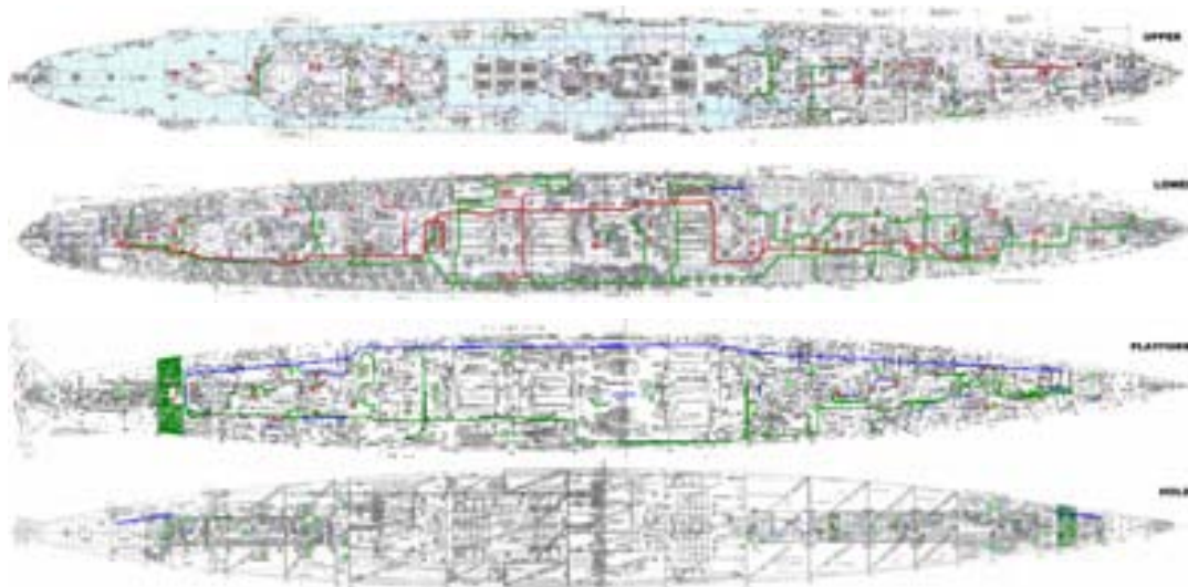
Figure 51: Fresh Water Service is indicated in green (the hot water is not shown); the Fresh Water Tanks are also marked in green. The thick red line indicates the saltwater or Main Service, and the thinner red line is the small bore feed to sanitary spaces. The Main Suction is indicated with blue lines.
