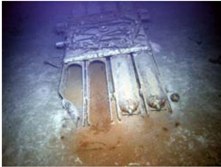
Figure 198: Port torpedo quad tubes containing two torpedoes [280]
