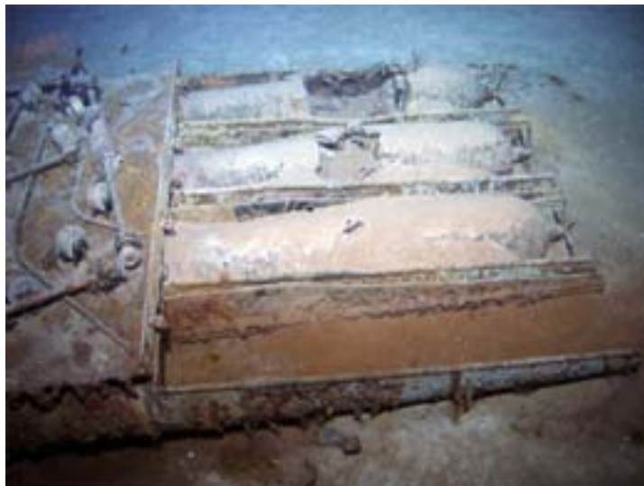
Figure 193: Starboard torpedo quad tubes showing damage to its three remaining torpedoes [277]
