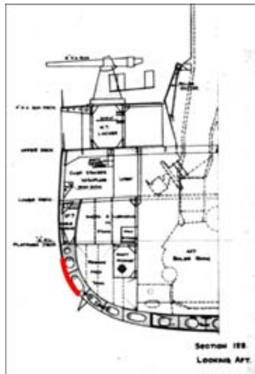
Figure 168: A section showing the extent of imploded or collapsed shell plating on the starboard side
