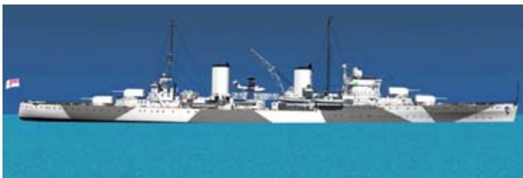
Figure 208: Sydney in calm water after sustaining damage due to torpedo hit. Note the reduced height from the tip of the bow to the waterline
