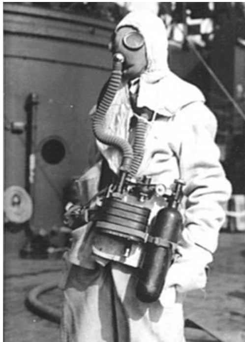
Figure 225: Salvus breathing apparatus (HMAS Australia, 1943) [299]
