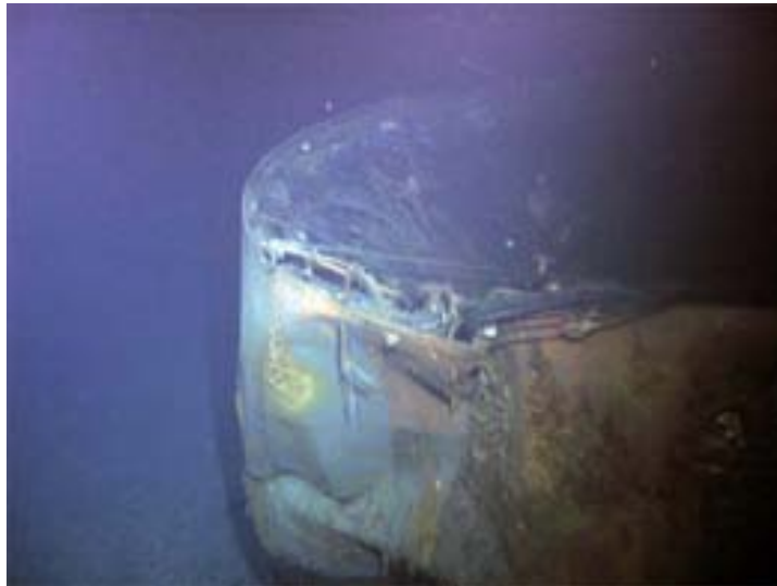
Figure 161: Collapsed structure at the stern of Sydney [255]
