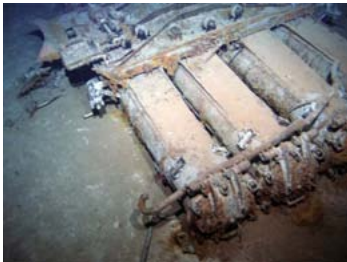
Figure 195: Starboard quad tube identified by the platform on the upper left hand corner of the photograph [278]
