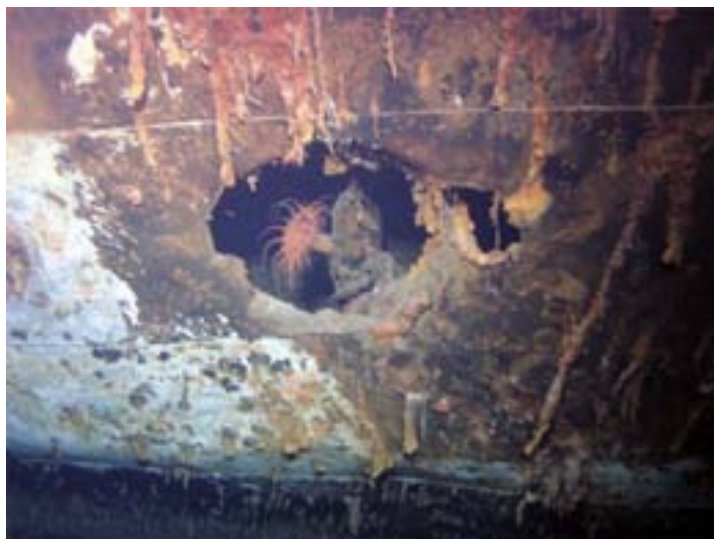
Figure 221: Example of contact detonating shell [294]
