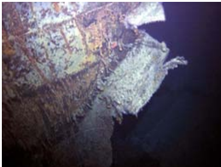
Figure 117: Flaring on the starboard side panels indicating that the torpedo either caused a hole or bulge on the starboard side [173]
