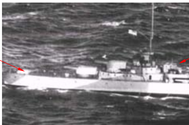
Figure 66: Sydney in August 1941 showing Carley floats on the stern and 2 vertical floats on the starboard side on the timber stowage rack [125].
