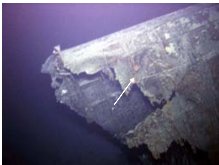
Figure 114: Break in bow on Port side showing indentation due to torpedo detonation [172]
