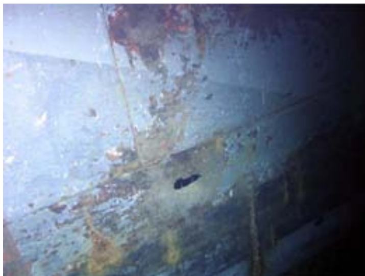
Figure 238: Example of a shell that has probably hit Sydney on an angle [309]
