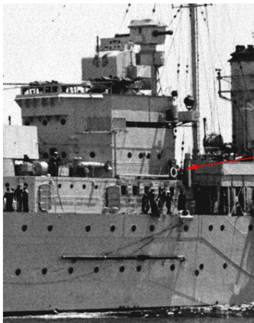
Figure 76: Photograph of Sydney port side showing single Kisbie lifebuoy on the forward superstructure [122].
