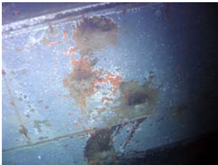
Figure 236: Non-penetrating shell damage to the armour plating [307]
