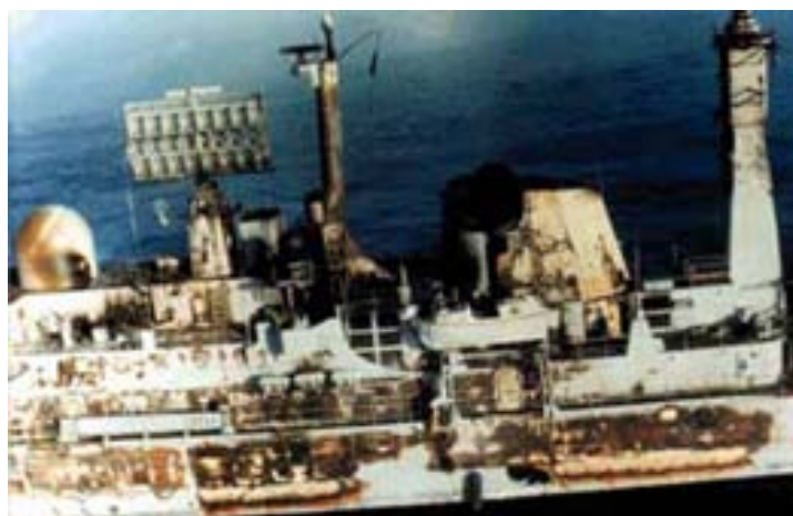
Figure 16: Fire damage to Sheffield [33]
