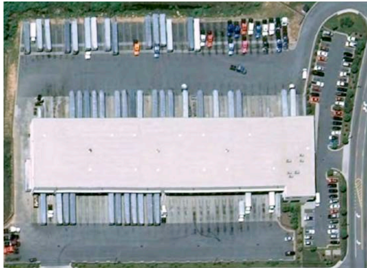
Figure 13.3: A typical crossdock is built in the shape of the letter I (actually, an elongated rectangle), so that freight can flow across from incoming trailers to outgoing trailers.
