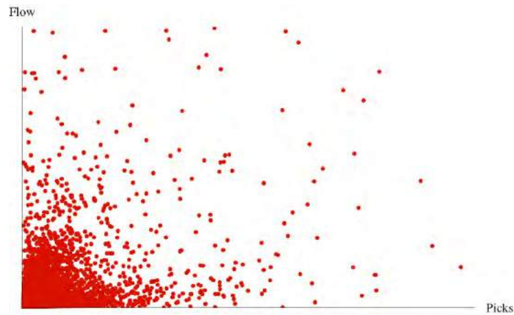
Figure 2.3: Among these 25,000 SKUs there is no correlation between popularity and physical volume of product sold.
