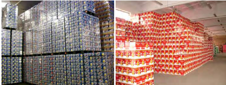
Figure 17.3: In the US warehouse on the left, cartons of beer have been palletized because labor is expensive compared to capital. The reduction in labor is worth the expense of a forklift plus the additional storage space. In the Chinese warehouse on the right, cartons have been stacked by hand and must be unstacked by hand; but labor is cheap and capital is expensive.
