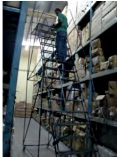
Figure 17.6: A ladder is much cheaper than a person-aboard truck, though much slower. (Note the product stored as loose cartons.)
