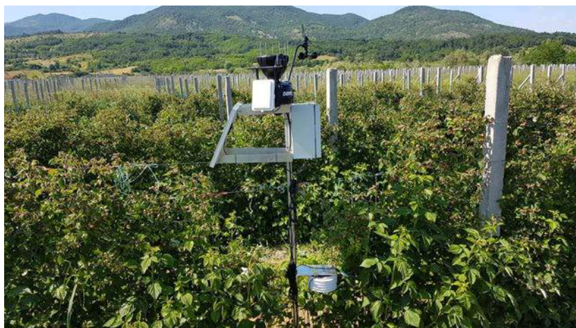
Figure 13.19: Agrometeorological weather stations in orchards for disease monitoring (Source: PFNS).
