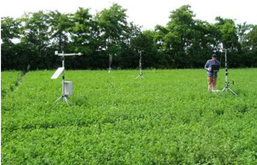
Figure 13.3: Transect measurements on wind and evaporation leeward of a hedgerow in Austria; (Source: BOKU-Met).
