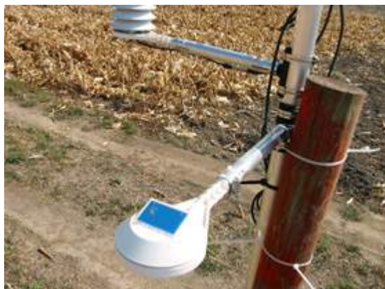
Figure 13.8: Leaf wetness sensor; (Source: BOKU-Met).
