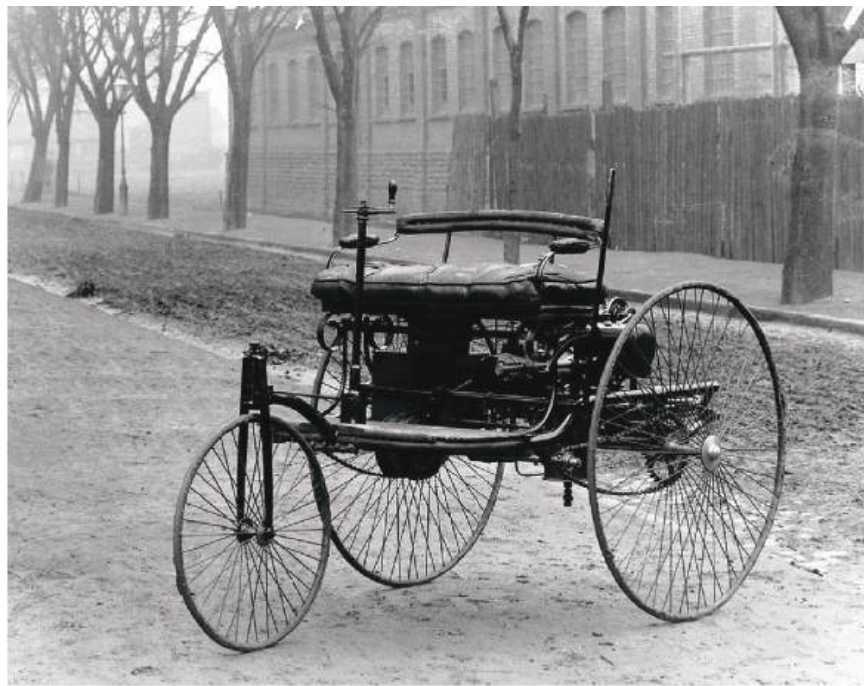
FIGURE 9.5 The First Automobile. This 1885 photo shows the Benz Patent-Motorwagen, the first automobile sold to consumers. It was a few more decades before automobiles came to resemble the cars we drive today. (credit: “1885 Benz” by Alonso de Mendoza/Wikimedia Commons, Public Domain)
