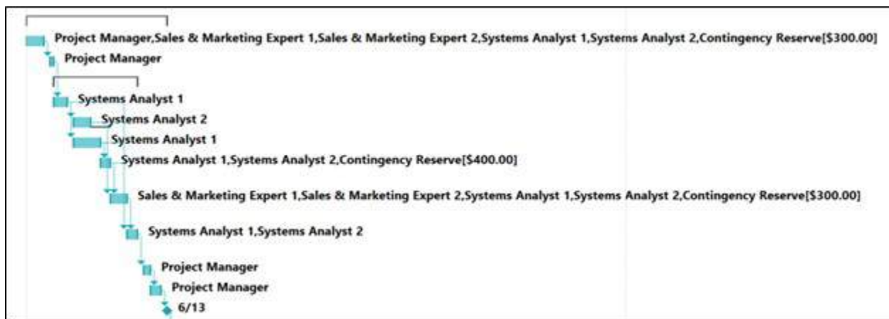
Figure 9.7: Gantt Chart with the resources indicated on the right of the bars
