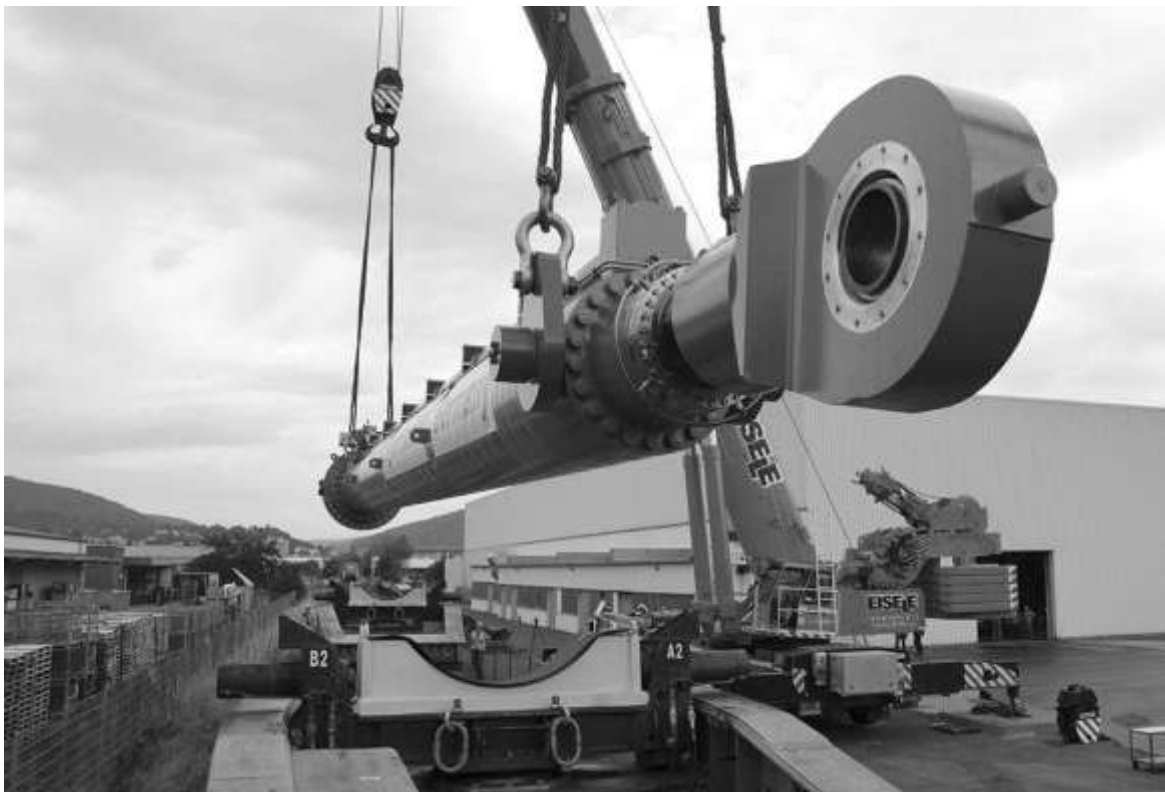
Figure 1-2 - Hydraulic Cylinder ( www.hunger-hydraulics.com )
