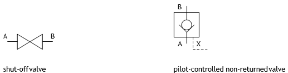
Figure 4-10 - Non-Return Valves (D.Merkle, M.Thomes and B.Schrader. Hydraulics Basic Level Textbook )
