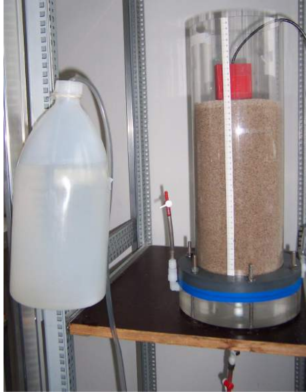
Figure 9.2: Overview of the measurement setup for the soil column
