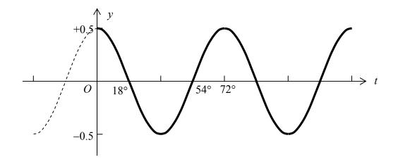
(viii) Amplitude = 0.5 , Period =  $72^{\circ}$  , Phase shift =  $-12^{\circ}$  (relative to basic cosine)
