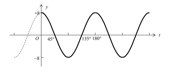
(vi) Amplitude = 8 , Period =  $180^{\circ}$  , Phase shift =  $20^{\circ}$  (relative to basic cosine)
