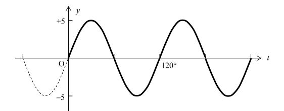
(ii) Amplitude = 5 , Period =  $120^{\circ}$  , Phase shift =  $15^{\circ}$  (relative to basic sine)
