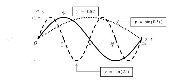
Multiplying the t inside the trig function by a constant stretches or compresses the basic wave-form horizontally, i.e. it alters the period and the frequency. In general, we obtain the following results:
