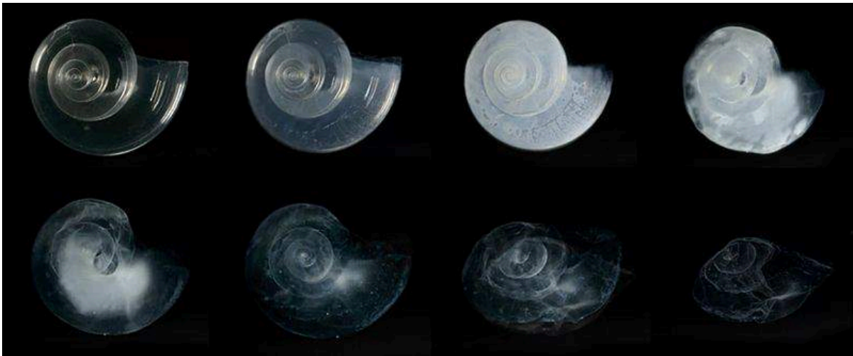
Figure 5.5.5 The results of an experiment placing the calcium carbonate shells of pteropods in seawater with a pH of 7.8, the projected ocean pH for the year 2100 under current rates of acidification. The top row shows the shells before the experiment, and the bottom row shows the dissolution of the shells after 45 days of exposure (NOAA).
