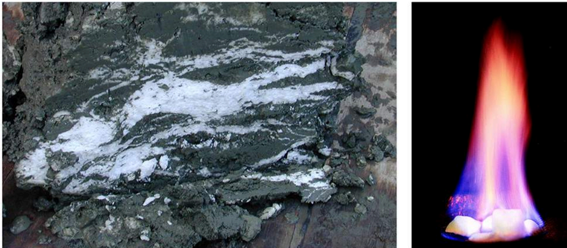
Figure 12.4.5 (Left): Methane hydrate within muddy sea-floor sediment from an area offshore from Oregon (By Wusel007 (Own work) [GFDL ( http://www.gnu.org/copyleft/fdl.html ) or CC BY-SA 3.0], via Wikimedia Commons). (Right): Methane hydrate on fire (USGS, http://www.usgs.gov/blogs/features/files/2012/01/New-Image.jpg ).
