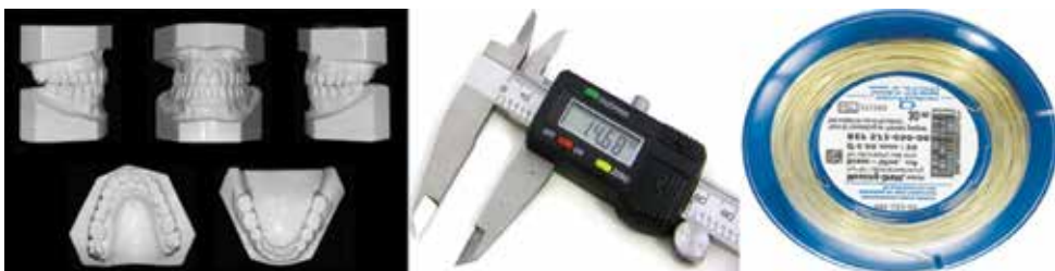
Figure 1. Plaster casts, digital Vernier caliper to performed all measurements and brass wire to measure arch length.
