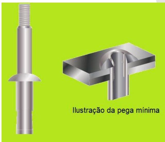
Fonte: FAA - Federal Aviation Administration - Mechanic Training Handbook Figura 6-40 Rebites Cherry-Lock Wiredraw.
