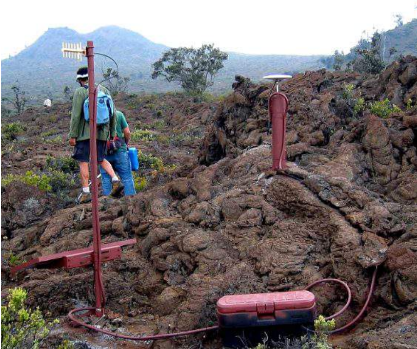
Figure 11.44 A GPS unit installed at Hualālai Volcano, Hawaii. The dish-shaped antenna on the right is the GPS receiver. The antenna on the left is for communication with a base station. Source: U. S. Geological Survey (n.d.) Public Domain
