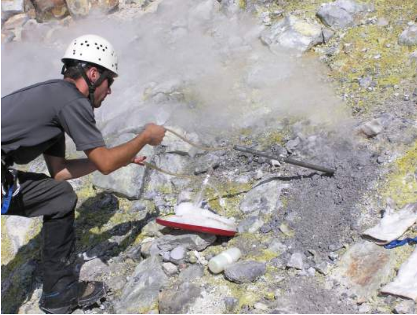
Figure 11.43 A geologist collects a gas sample from Sherman Crater, Mt. Baker, Washington. Gas is drawn through a titanium tube inserted in a fumarole, and collected in a glass vacuum flask. Source: D. Tucker, U. S. Geological Survey (2006) Public Domain
