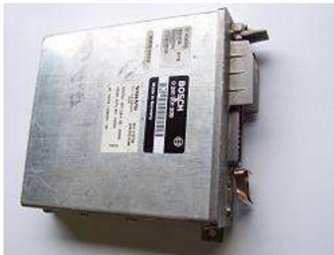
EDC control unit
