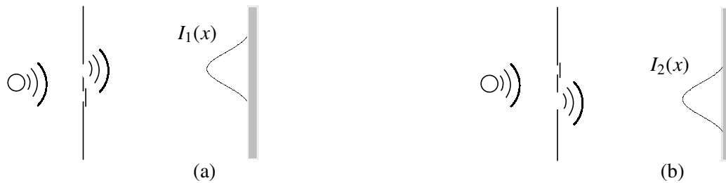
Figure 4.4: The result of directing waves at a screen when only one slit is open. The curves I_1(x) and I_2(x) give the intensities of the waves passing through slit 1 or 2 respectively and reaching the screen at x . (They are just the central peak of a single slit diffraction pattern.)
