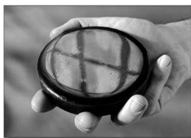
Test glass produced by vitrification process.
