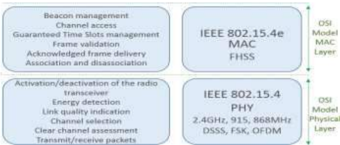
Figure 3.10 IEEE 802.15.4 compared with OSI reference model.
