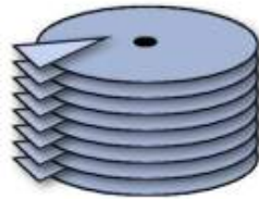
Figure 13: Platters in a HDD
