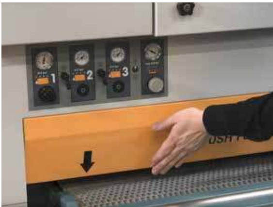
Safety switch stops dangerous moving parts when you open hatches.
