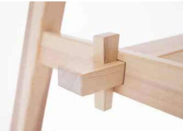
A keyed mortise and tenon joint is good for easy assembly. In this case the tenon goes through the leg and is wedged on the outside. Design Hemmo Honkonen, Malmstens, Linköping University.
