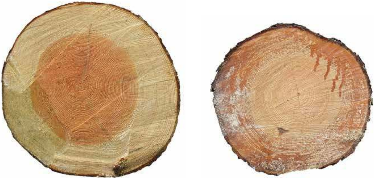
These pine logs were recently felled. The left image shows the root end and the extent of the pine heartwood. The right image shows the top end and how the transport of nutrients, in the fluid which runs through the sapwood in the log, has not yet stopped.
