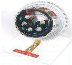
Fig: Cutaway Model Of Multi-Plate Clutch
