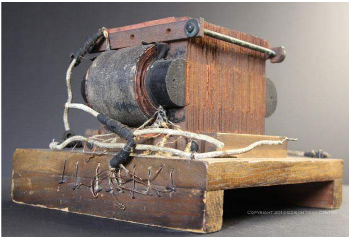
The original 1885 Stanley prototype transformer at the Berkshire Museum .
