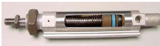
(b) Cross section of a single acting cylinder
