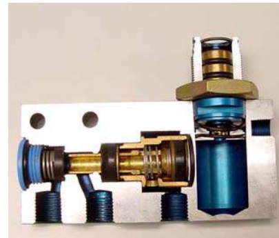
(b) Cross section of a 3/2 directional control valve
