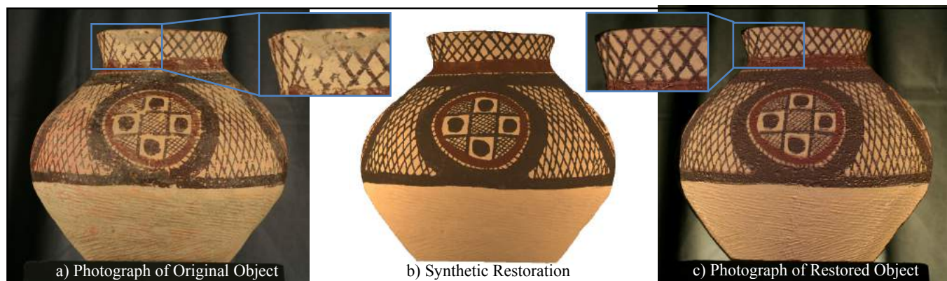
Figure 1. Virtual Restoration. We present a system to restore and alter the physical appearance of old and deteriorated objects: a) photograph of an ancient Chinese vase (ca. 2250 BC); b) an image of the synthetic restoration produced by our algorithm; c) photograph of the restored object using our system and guaranteed not to exceed a provided maximum amount of light per unit surface area (note: in photographs, background is illuminated by a light source behind the object causing shadows on the rim of the object).
