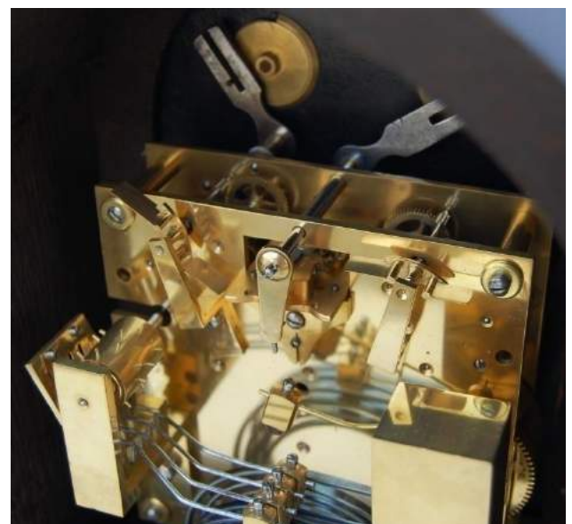
Figure 31 – another view (note the platform escapement mounted between the plates)
