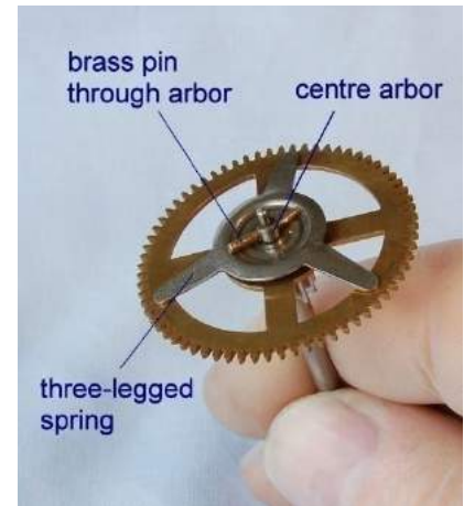
Figure 90 – the components of the friction drive
