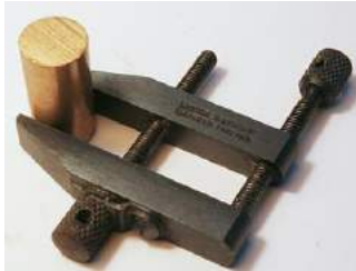
Figure 143 – a toolmaker's clamp
