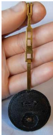
Figure 53 – a mantel clock pendulum
