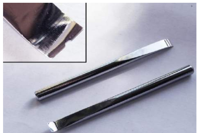
Figure 147 – Hand removing levers made by students. Both show a few imperfections and slight dimensional inaccuracies, but are nevertheless very good examples. Note the overall geometry of the tip curve (bend) is better in the left hand example; in the right hand example the curve is continuous right to the tip.
