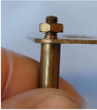
Figure 98 – pillars fastened to plates with nuts
