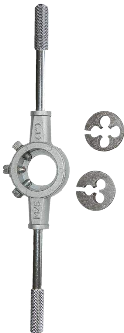
Figure 133 – die stock and two dies
