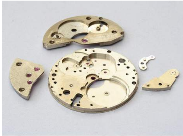
Figure 57 – example watch plate, bridges and cocks
