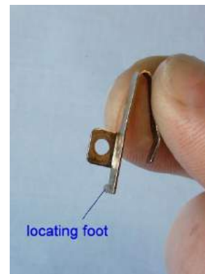
Figure 75 – detail of click spring
