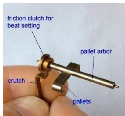
Figure 69 – pallet assembly
