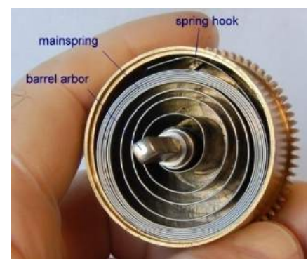
Figure 84 – barrel with end cap removed
