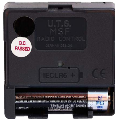
Figure 42 – radio controlled quartz movement
