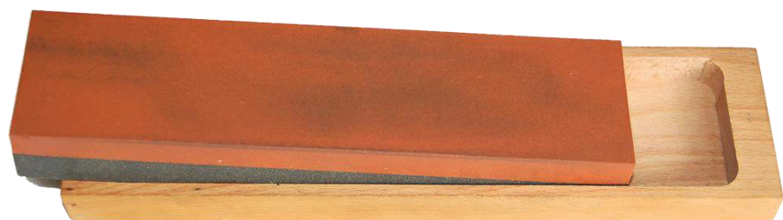
Figure 135 – India (aluminium oxide) stone
