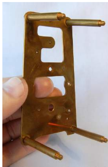
Figure 94 – front plate with pillars
