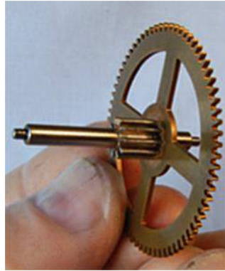
Figure 85 – intermediate wheel and pinion
