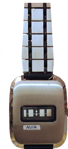
Figure 50 – very early LCD watch with "random dispersal" display
