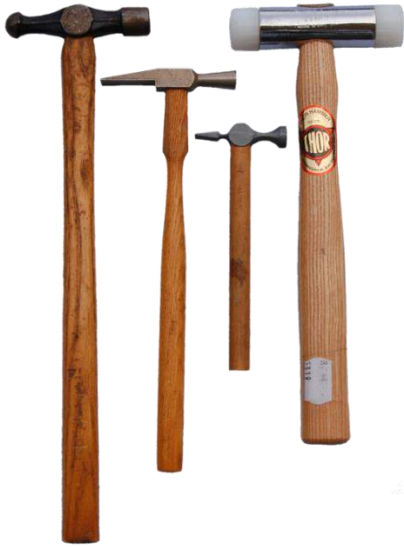
Figure 117 – from left to right: ball pein hammer; clock hammer; watch hammer; soft nosed hammer
