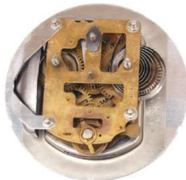
Figure 34 – movement of Smith alarm clock
