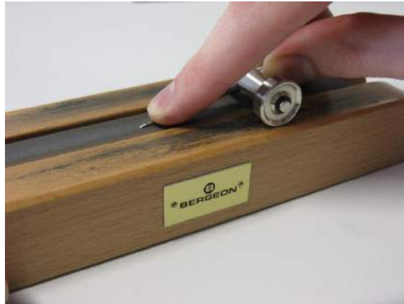
Figure 109 – using a screwdriver sharpening device
