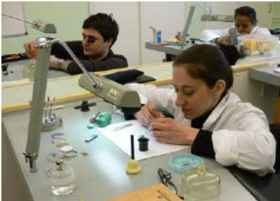
Figure 3 – a watchmaker’s bench. Note the adjustable lamp and height of the bench, both of which facilitate comfortable working
