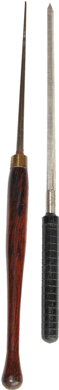
Figure 131 – smoothing broach (left), and cutting broach
