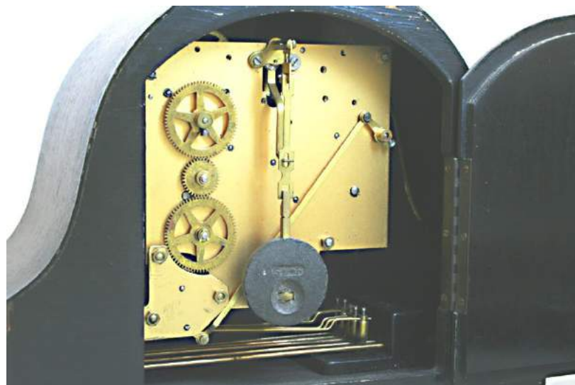
Figure 26 – rear view of chiming mantel clock showing gongs and hammers
