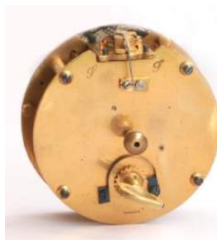
Figure 20 – drum movement showing platform escapement
