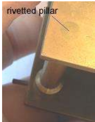
Figure 99 – pillar rivetted to back plate
