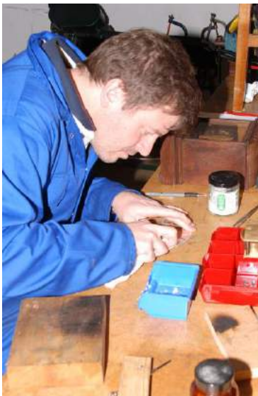
Figure 10 – silvering a chapter ring in the BHI clock workshop
