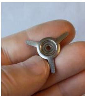
Figure 91 – three-legged friction spring
