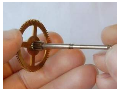
Figure 92 – centre arbor in the centre pinion
