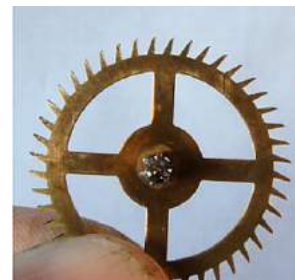
Figure 88 – tooth form of escape wheel
