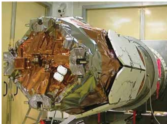
Figure 1. Offtek satellite top plate with monopropellant hydrazine thrusters [2].
