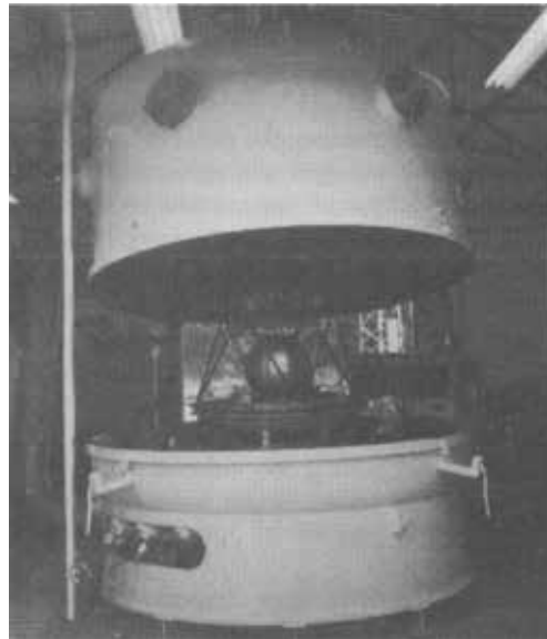
Figure 7. Entire system EM testing vacuum chamber [1].
