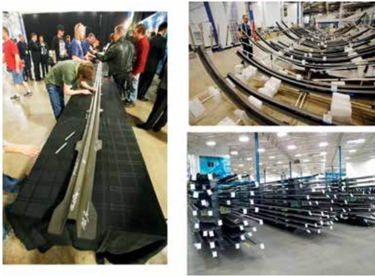
Figure 36. A350 precured omega stringers. Source: Deseret News, Jeffrey D. Allred; CW/Photos: Jeff Sloan.
