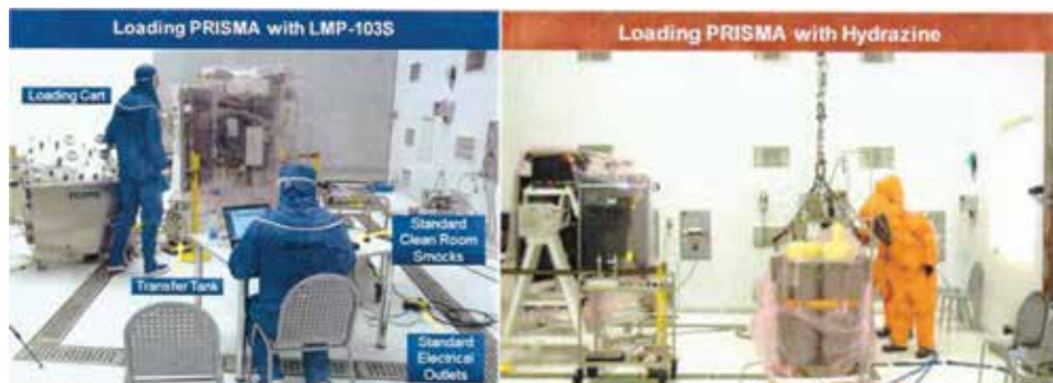
Figure 8. Propellant loading of satellite Prisma [20].
