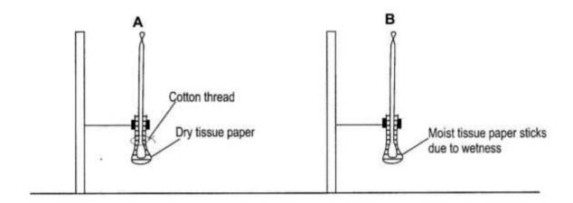
Wrap the bulb of thermometer **B** with moist tissue paper. Thermometer **A** is already wrapped for you with a similar amount of dry tissue.
