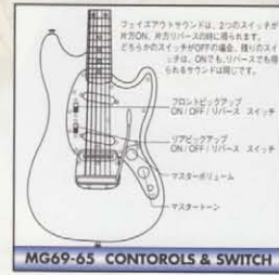
MG69-65 CONTROLS & SWITCH
