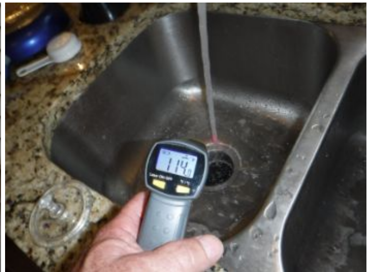
Water Temp (reading)- The water temperature at faucet is reading 110-115 degrees which is considered hot.
