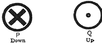
FIG. 2.—Direction of an electric current.
