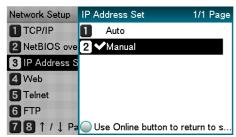
When obtaining an IP address automatically, confirm that [Auto] is selected, and then press the <OK> button.
