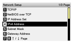
Press the scroll buttons ▲ and ▼ or the numeric keypad to input the first three digits of the IP address, and then press the <OK> button. Use the same operation to input the next three digits. After input is complete, press the <BACK> button.
