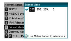
Press the scroll button ▼ to select [Gateway Address], and then press the <OK> button.
