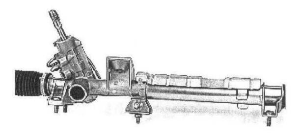
Transfer the mounting for the center mounting. Plug the open ends of pipe couplings.
