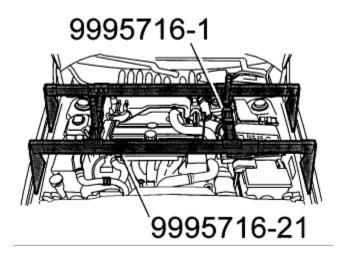
Connect brackets 999 5716-21 and 999 5716-land lifting hooks 999 5460-21. Lift the engine to relieve the load on the engine pads.
