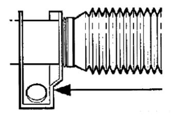
Check that the <u>tie rod</u> is in the same position as when it was removed.
