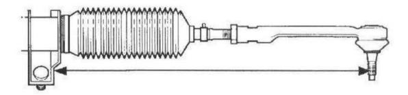
On one side, measure the length of the  $\underline{\text{tie rod}}$  relative to the steering gear housing. Note the measurement
