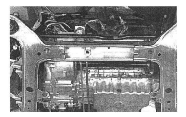
Lift the steering gear in from the right.
