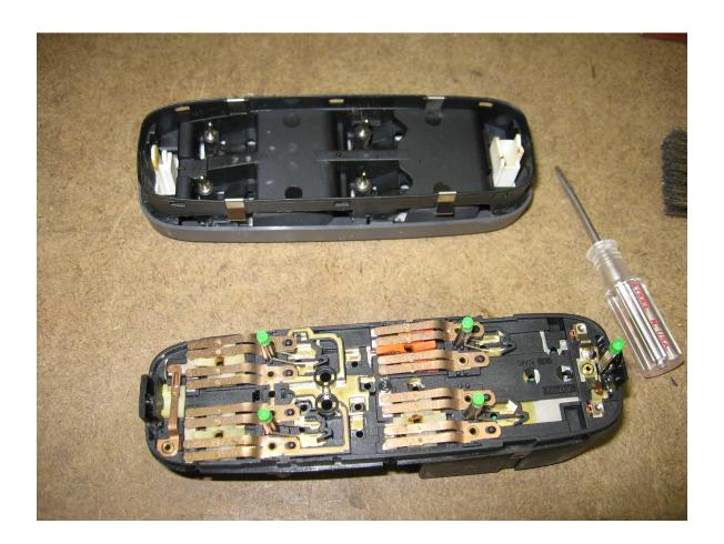
Once you get it back together check all retaining clips and put the plugs back in. Then test it.
