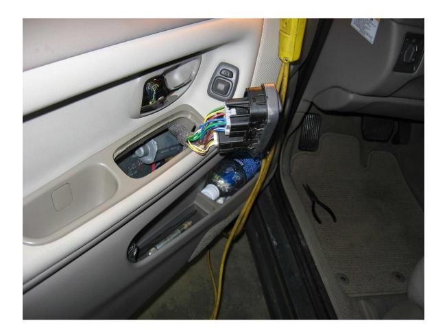
Gently remove the wiring harness plugs; the clips holding them in place can be disengaged with a minimum of effort. Try not to pull on the wires but grasp the plug itself. The white one was the hardest due to the retaining clip being right next to the circuit board box.
