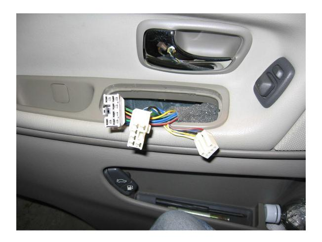
Recommend tools. Note the compartment on right where the smallest plug goes. Unless there is a lot of dirt, it is probably not necessary to take this apart as there is only a circuit board in there. See the next picture.
