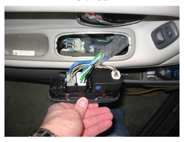
Look for dirt accumulation. Clean the ridges around the opening, vacuum if necessary.
