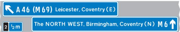
The panel with the inclined arrow indicates the destinations which can be reached by leaving the motorway at the next junction
