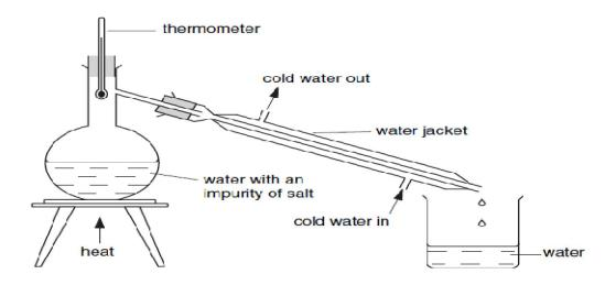
As the solution boils, the water in it evaporates as water vapour. The cold water flowing through the condenser cools the steam passing the delivery tube (water jacket). The steam condenses back to liquid which drips in to the collecting beaker. The liquid collected in the beaker is called the distillate and is pure water.
