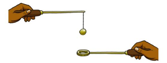
Before heating, an iron ball can pass through the ring.
