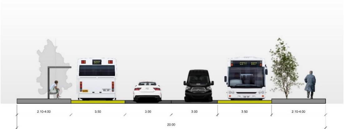
Figure 41: Cross section: two-way road with bus lanes 2 directions
