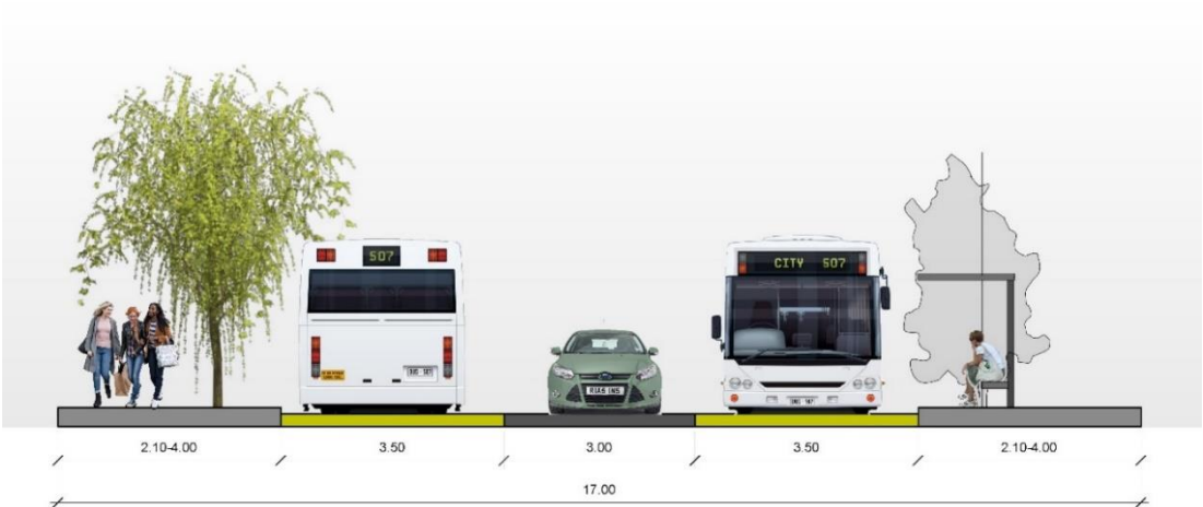
Figure 42: Cross section: one-way road with separate bus lanes 2 directions
