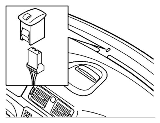
Lift up the sun sensor. Disconnect the connector. Remove the sun sensor.
