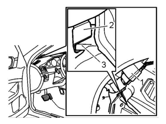
Pull the dashboard back slightly so that the brackets for the connectors at the A-post can be removed.
